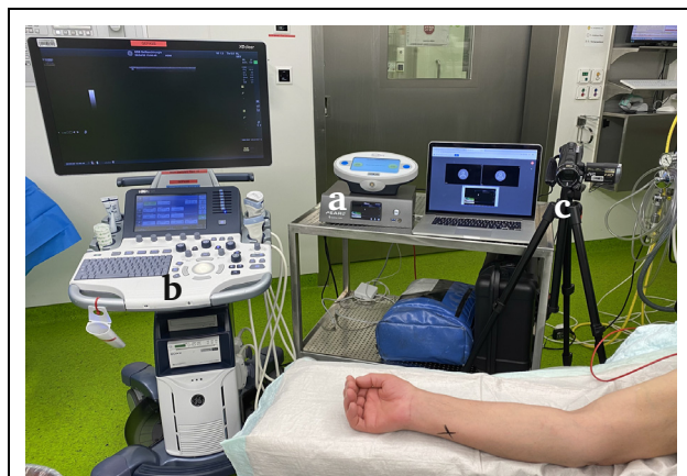
Figure 1. Teleproctoring device setup with Pearl-2, Epiphan video encoder (a) connected to GE Logiq S8 ultrasound (b), and HD video camera (c) via HDMI for percutaneous ultrasound guided creation of an arteriovenous fistula for haemodialysis access.
