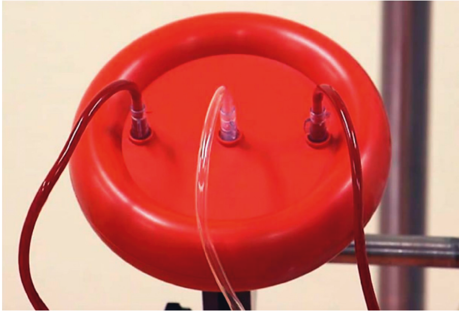
FIGURE 1: The HemoClear device at work. Shed blood enters the filter from the left inlet and is separated into concentrated RBCs that leave the filter from the right outlet and plasma that flows away in the middle outlet.
