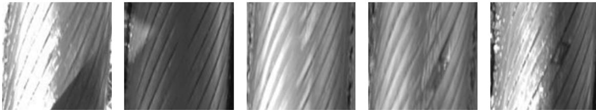
**Figure 3.** Real samples of wire rope images captured from hauling ropes.
