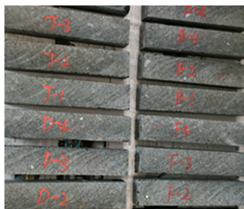
Figure 7. Samples of Four-point Bending Fatigue test.
