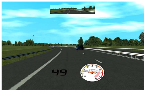
Fig. 2. The central monitor view of the driving environment with rear-view mirror and digital speedometer displayed. A DRT target is presented above the horizon on the left.
