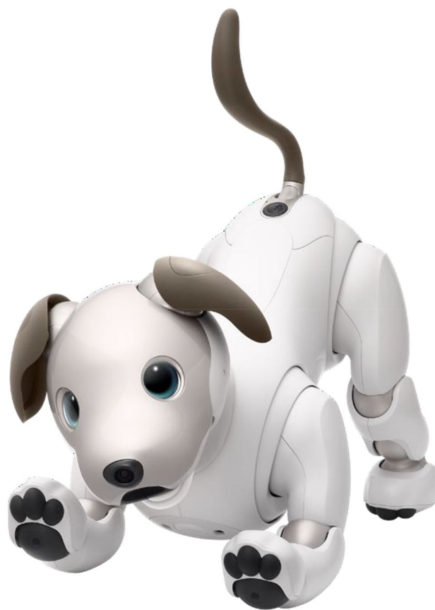
Fig. 1 aibo. Specification. Product name: aibo, model number: ERS-1000, processor: 64 bit quad-core CPU, display: 2 OLEDs (eyes), sound: speaker, 4 microphones, camera: 2 cameras (front camera, SLAM camera), communications: mobile network communication feature (data transmission) LTE, Wi-Fi IEEE 802.11 b/g/n (2.4 GHz), outside dimensions: approx. 180×293×305 mm, weight: approx. 2.2 kg, power consumption approx. 14 W, battery duration: approx. 2 h, recharge time: 3 h
