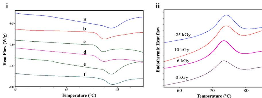
Fig. 5. DSC results of starch. i. DSC thermogram of native and irradiated kithul starch (a) 0 kGy, (b) 0.5 kGy, (c) 1 kGy, (d) 2.5 kGy, (e) 5 kGy, (f) 10 kGy. Figure adapted with permission from Sudheesh et al. (2019). ii. DSC gelatinization endotherm of native (0 kGy) and irradiated (6, 10, 25 kGy) sago starch. Figure adapted with permission from Othman et al. (2015).
