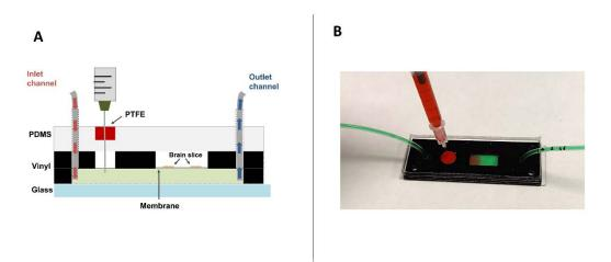
**Figure 2.** (**A**) Schematic diagram flow of the brain slice-on-a-chip. Hippocampal brain-slices rest over the PC membrane, whereas the culture medium and the OGB solution are perfused across the lower compartment. (**B**) A real injection test replicates Figure 2A. Green fluid is perfused in the lower chamber, and the red fluid is injected through the PTFE plug in the pre-chamber.
