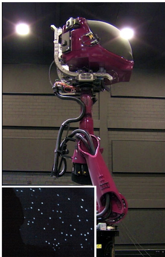
Fig. 1 Experimental setup. Participants sat inside the simulator cabin and were presented with visual stimuli projected on the inner surface of the cabin door. The inset provides a picture of the visual stimulus
