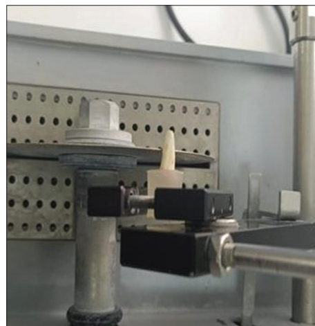
Figure 1: Sectioning the samples using microtome
