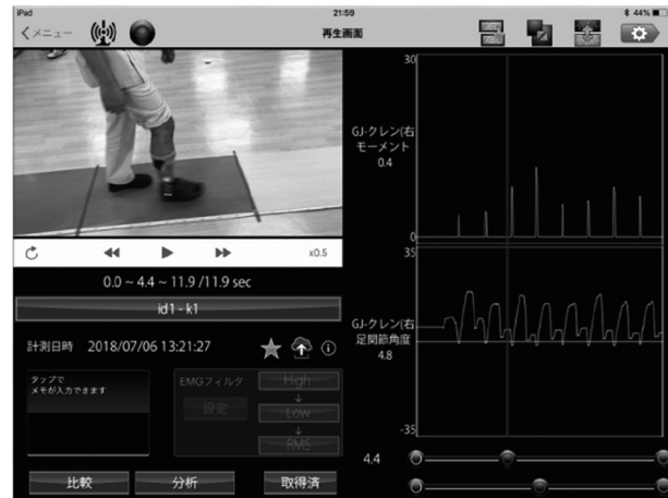
Fig. 2. PFRTs and angles of the ankle joint are displayed graphically synchronized with the video tracked at the measurement.
