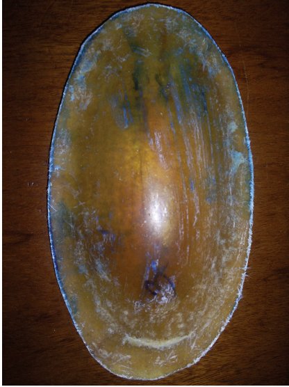
FIGURE 5: Composite hip protector with three layers on the reinforced shell.
