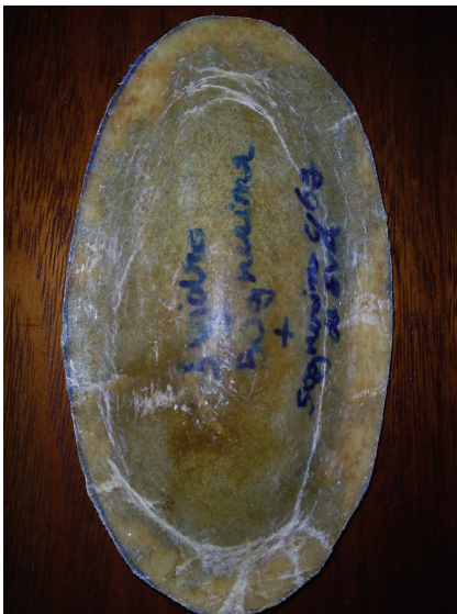
FIGURE 6: Hip protectors fabricated with one layer of glass fiber chopped strand mat and gel coat with EVA particles content of 10 wt. %, after impact load.
