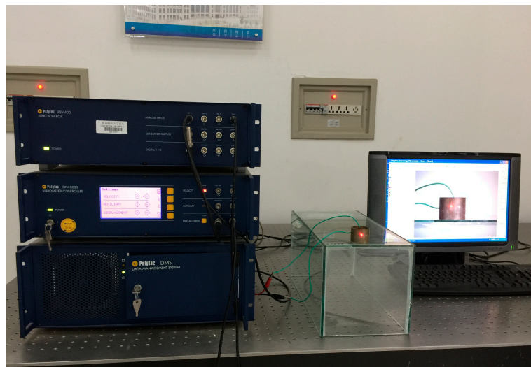
Figure 6. Experimental setup for the measurement of the radially polarized piezoelectric cylindrical transducer.
