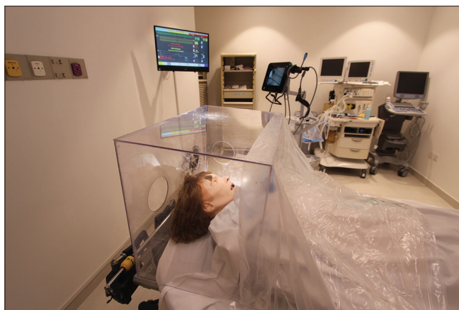
Figure 1: Modified aerosol-box barrier placed on manikin
