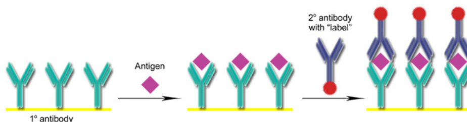
Fig. 4. Schematics of “Sandwich” type immunoassay.
