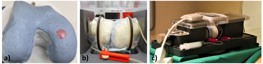
Figure 5. Device for the standardized, displacement-controlled compressive loading of human articular chondral samples. In preparation of this study, an intact right human knee joint had been scanned by CT to obtain the bone contours of femur and tibia which were 3D printed and subsequently covered by wiroasil ® silicone (as artificial cartilage layer) in its native configuration. (a) At the center of the medial femoral condyle a circular defect (8 mm diameter, 3 mm depth) was created within the wiroasil ® silicone (blue material) to be filled with native human articular cartilage samples of equal dimensions (red). (b) Loading was brought about by axial displacement of the tibial component (left) against the fixed femoral component (right). The standardized knee was covered by a transparent artificial joint capsule sealed with O-rings and filled with PBS buffer. (c) The assembled and sample-loaded device is displayed within the bore of a 3.0 T MRI system; for imaging, a dual-coil setup was used (attached above and below the knee).
