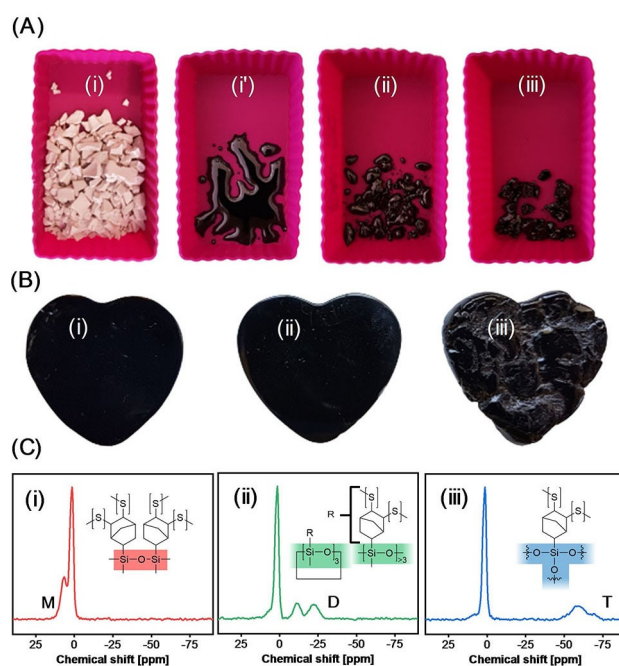
Figure 1. A) Melting behavior of branch -poly(S- r -NBS 20 ) with different degree of siloxane branching. Granules of branch -poly(S- r -MENBS 20 ) before (i) and after 2 h (i') at 80 °C. Granules of (ii) branch -poly(S- r -DCNBS 20 ) and (iii) branch -poly(S- r -TCNBS 20 ) after 2 h at 80 °C. B) Molded objects made from 2 g of branch -poly(S- r -NBS 20 ) at 80 °C overnight. While (i) branch -poly(S- r -MENBS 20 ) and (ii) branch -poly(S- r -DCNBS 20 ) adopted the shape of the mold, branch -poly(S- r -TCNBS 20 ) was still rubbery at 80 °C and did not fully adopt the shape of the mold. C) 29 Si CP/MAS NMR spectra of (i) branch -poly(S- r -MENBS 20 ), (ii) branch -poly(S- r -DENBS 20 ), and (iii) branch -poly(S- r -TENBS 20 ), showing characteristic peaks for M, D, and T siloxane bonds, respectively. The peak at 1.4 ppm present in each of the spectra corresponds to the trimethyl-substituted silicon atom stemming from the TMNBS comonomer.
