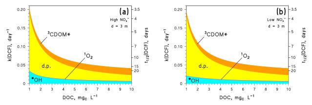
**Figure 5.** Modelled first-order degradation rate constants (k(DCF)) and half-life times ( $t_{1/2}$ (DCF)) of DCF, as a function of DOC. Assumed water conditions: d = 3 m,  $[HCO_3^-] = 10^{-3}$  M and  $[CO_3^{2-}] = 10^{-5}$  M, plus (**a**)  $[NO_3^-] = 10^{-4}$  M,  $[NO_2^-] = 10^{-6}$  M, or (**b**)  $[NO_3^-] = 10^{-6}$  M,  $[NO_2^-] = 10^{-8}$  M. The importance of different photoreaction pathways is highlighted with different colours (d.p. = direct photolysis).
