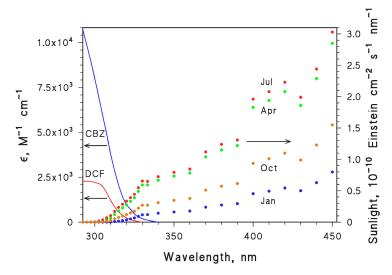
**Figure 7.** Left *y*-axis: Absorption spectra (molar absorption coefficients  $\varepsilon$ ) of CBZ and DCF. Right *y*-axis: Spectral photon flux density of sunlight at 45°N latitude, in the months of January, April, July and October (15th day of each month).
