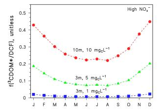
**Figure 6.** Modelled fraction of DCF phototransformation accounted for by  $^3$ CDOM\* (f( $^3$ CDOM\*/DCF)), in the different months of the year (45° N latitude, fair weather) and for different values of water depth (d=3 or 10 m) and DOC (1, 5 or 10 mg<sub>C</sub> L $^{-1}$ ). In all cases, high NO<sub>X</sub> $^-$  conditions ( $10^{-4}$  M nitrate,  $10^{-6}$  M nitrite), [HCO<sub>3</sub> $^-$ ] =  $10^{-3}$  M and [CO<sub>3</sub> $^2$ ] =  $10^{-5}$  M were assumed.
