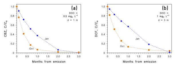
**Figure 4.** Time trends of (a) CBZ and (b) DCF, in the months following emission (the month of emission is highlighted). Assumed water conditions:  $[NO_3^-] = 10^{-4} \text{ M}$ ,  $[NO_2^-] = 10^{-6} \text{ M}$ ,  $[HCO_3^-] = 10^{-3} \text{ M}$  and  $[CO_3^{2-}] = 10^{-5} \text{ M}$ , plus (a) DOC = 0.5 mg<sub>C</sub> L<sup>-1</sup>, d = 1 m, or (b) DOC = 1 mg<sub>C</sub> L<sup>-1</sup>, d = 3 m. Data points are connected by linear segments as a guide to the eye.
