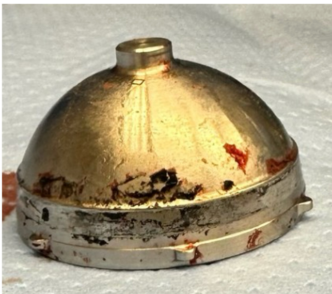
Figure 2. Explanted CoCrMo liner with a polar centralizing post and macroscopically visible dark corrosion products at and around the equatorial locking taper. CoCrMo, cobalt chrome alloy.
