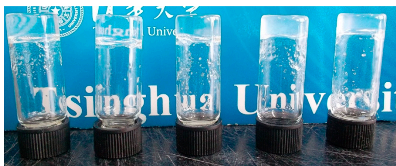
Figure 1. Gels in chloroform/toluene, chloroform/ p -xylene, o -dichlorobenzene, bromobenzene, chlorobenzene (from left to right).
