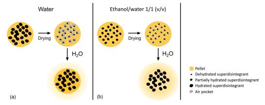
**Figure 3.** Schematic representation of the influence of the pelletizing liquid during the production process on the disintegration behavior of the pellet in aqueous dissolution media. (a) Water as a pelletizing liquid leads to air pockets in the dried formulation hampering disintegration during dissolution; (b) ethanol/water 1/1 (v/v) as a pelletizing liquid leads to smaller air pockets in the dried formulation enabling disintegration during dissolution.
