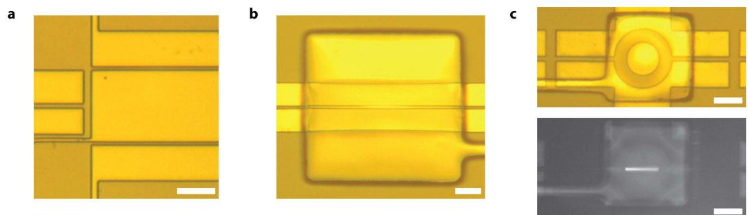
Figure 5. Example PDMS Waveguide Platform Microscope Images. (a) Reconfigurable optofluidic MMI, empty; (b) Lightvalve in its static state, empty; and (c) Lightvalve trap, both empty (top) and filled and under optical excitation (bottom). The filling fluid for the lightvalve trap is a 3\ \mu\text{M} Dylight 488 solution and exhibits fluorescence when excited by 488 nm laser light, injected from the left solid-core waveguide. Note: all white scale bars represent 50\ \mu\text{m} .
