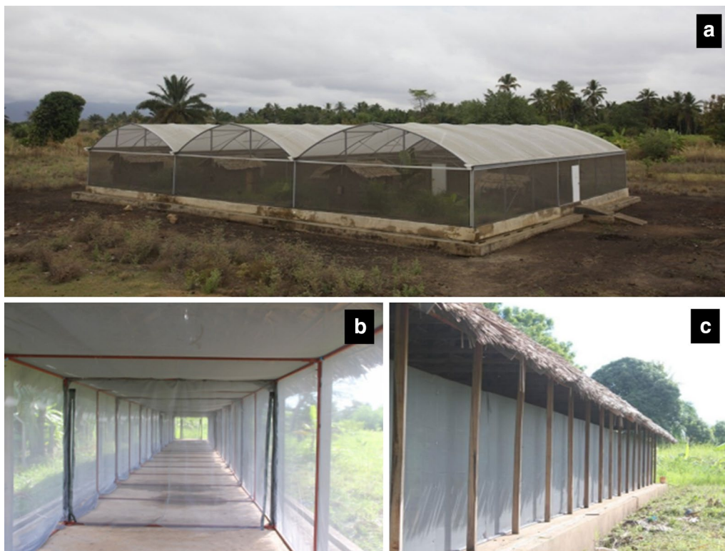
Fig. 1 The semi-field systems used for the experiments. a shows the large multi-compartment system; b shows the inside sections of the long tunnel-shaped, semi-field system; c is an outside view of the long tunnel-shaped semi-field system
