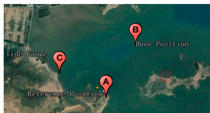
Figure 9. The location of study area near Qingdao, China. A is the fixed reference GPS station, B is the multi-function buoy, and C is the long-term tide gauge station.
