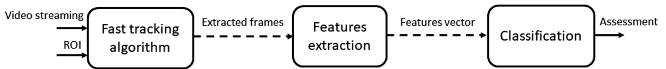
Figure 1. Block architecture of the proposed algorithm. Three main blocks are outlined: (i) a fast tracking algorithm to track the selected ROI, (ii) a feature extraction block to pre-process the available frames and (iii) a ML-based classifier to provide the output in terms of quality of perfusion.
