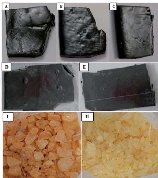
Fig. 1 Analysed samples (A, B, C) and standards (D and E) containing curing resin I and II.
