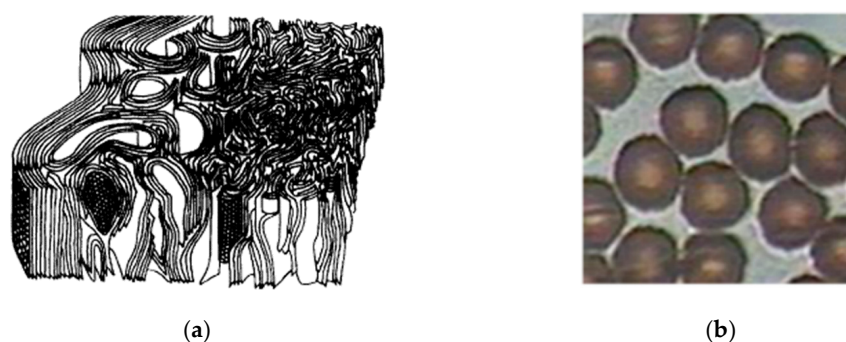
Figure 1. Skin-core structure of PAN fiber of (a) skin-core structural model of carbon fiber [10] and (b) micrograph of skin-core structure of pre-oxidized fiber [12].
