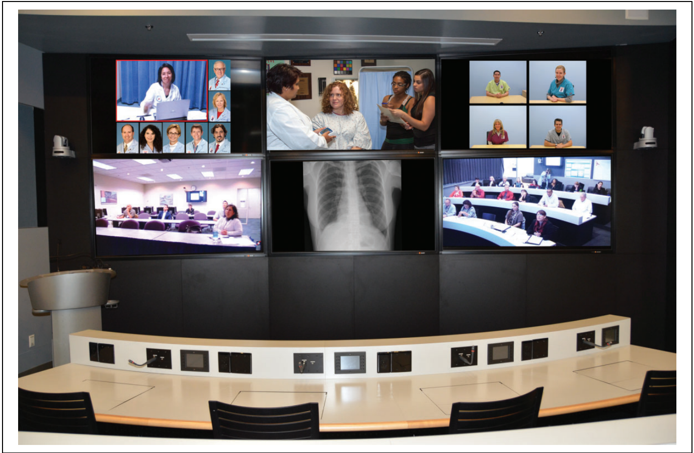
Figure A2. Video wall in the Arizona Telemedicine Program’s T-Health Amphitheater in downtown Phoenix, Arizona. This was created by Dr. Ronald S. Weinstein and his team of computer specialists. His ATP staff programmers, and outside contractors, worked on the customized computer software packages for the video wall implementation for nearly five years. Dr. Weinstein managed the project from Tucson. The T-Health Amphitheater (“e-Classroom-of-the-Future”) received the first place 21st Century Achievement Award, education facility category, in the International ComputerWorld Honors program, in 2008. Six 80-inch video screens, comprising a 7 foot \times 18 foot video wall. This dual-function videoconferencing facility was designed as a “command and control” center for Interprofessional Education and Collaborative Practice (IPECP) distributed training and as content aggregator and dissemination center for an envisioned statewide K-12 student medical science education program. Video wall; upper left, 8 off-campus faculty member participating in the video conferenced classroom session; lower left, off-site Tucson participants in the video conference; upper right, “stacks” of off-campus students participating in the video conference, each “stack can accommodate up to 50 students, waiting in a queue to move to the front of the stack, by voice activation. Individual stacks could be constituted of 7th grade, 8th grade, 9th grade, and 12th grade students respectively; lower right, Phoenix participants in the video conference (they could be members of the lay public auditing a student session); upper middle, patient being worked up at a rural clinic in the Arizona Telemedicine Network; lower middle, chest X-ray of a patient (simulation).
