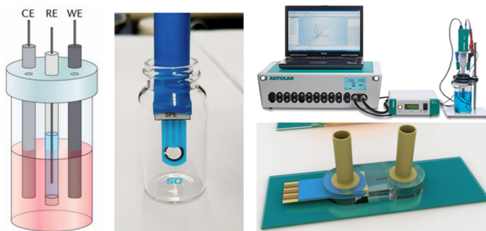
FIGURE 2 A typical experimental setup showing the reference, counter, and working electrodes (left); setup employed for in-lab experiments with SPEs (middle); Metrohm Autolab N series potentiostat (top-right); design of a flow-through environment using a membrane-based lab-on-chip sensor system (bottom-right)
