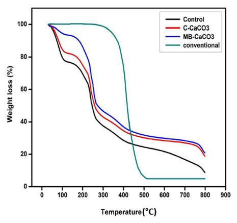
**Figure 6.** Thermogravimetric analysis (TGA) curves of control, commercial calcium carbonate (C–CaCO<sub>3</sub>)-based red seaweed (*Kappaphycus alvarezii*), microbially induced precipitated calcium carbonate (MB–CaCO<sub>3</sub>)-based red seaweed (*Kappaphycus alvarezii*), and conventional films [83].
