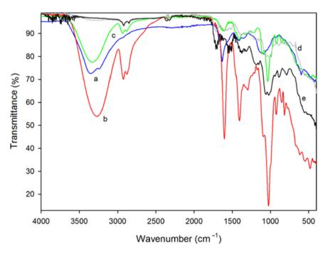
**Figure 5.** Fourier transform infrared spectroscopy attenuated total reflection (FTIR-ATR) spectrum of the (a) *C. tomentosum* seaweed extract (blue) and the different tested films: (b) 1% alginate (red), (c) 1% alginate with 0.5% of *C. tomentosum* seaweed extract (green), (d) 1% chitosan (grey), and (e) 1% chitosan with 0.5% of *C. tomentosum* seaweed extract (black) [78].
