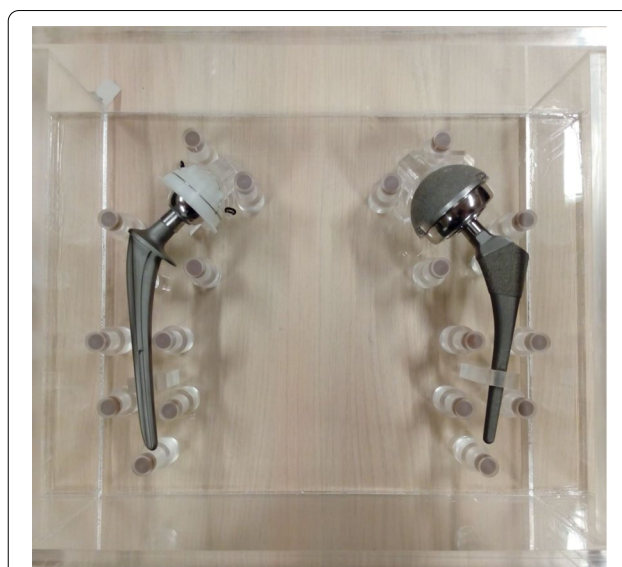
Fig. 1 Image of the phantom containing bilateral prostheses at the right (cup: UHMWPE, head: ZTA, stem: CoCrMo) and left (cup: CoCrMo, head: CoCrMo, stem: TiAlV). UHMWPE ultrahigh molecular weight ethylene, ZTA Zirconia toughened aluminum, TiAlV titanium–aluminum–vanadium, CoCrMo cobalt–chrome–molybdenum
