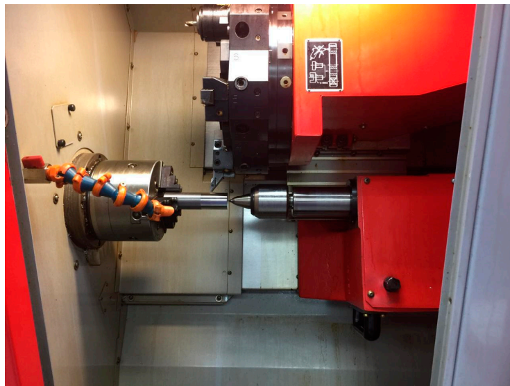
Figure 1. Test rig used for high-speed machining of Ti-6Al-4V.
