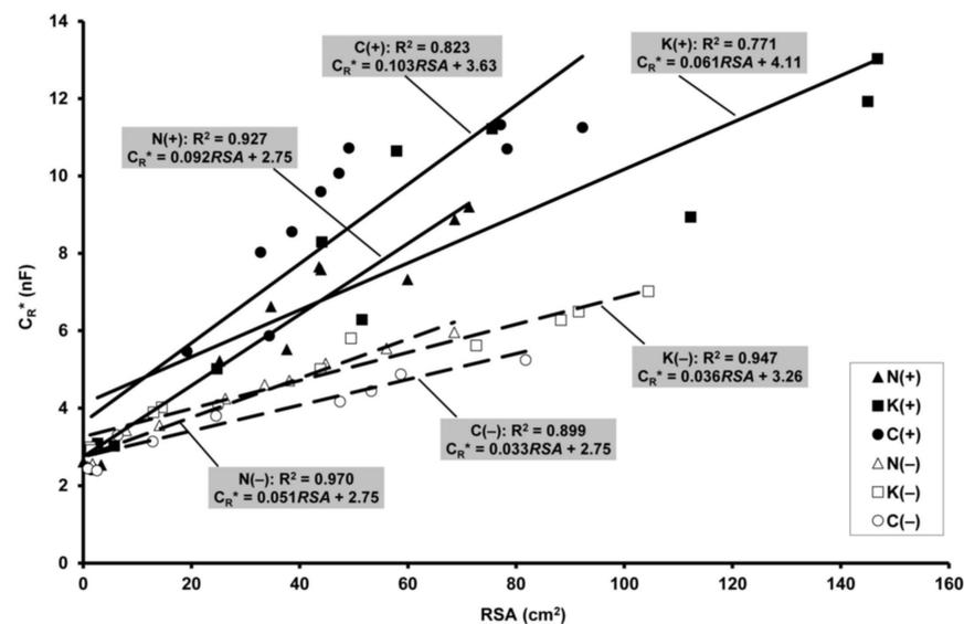
**Figure 6.** Linear relationships between the apparent root electrical capacitance ( $C_{R^*}$ ) and root surface area (RSA) in well-watered (filled symbols and solid lines) and drought-stressed (empty symbols and dashed lines) treatments. Only data obtained up to the flowering stage of the wheat genotypes were considered, and were pooled over the two pea treatments. For treatment codes, see Figure 1.
