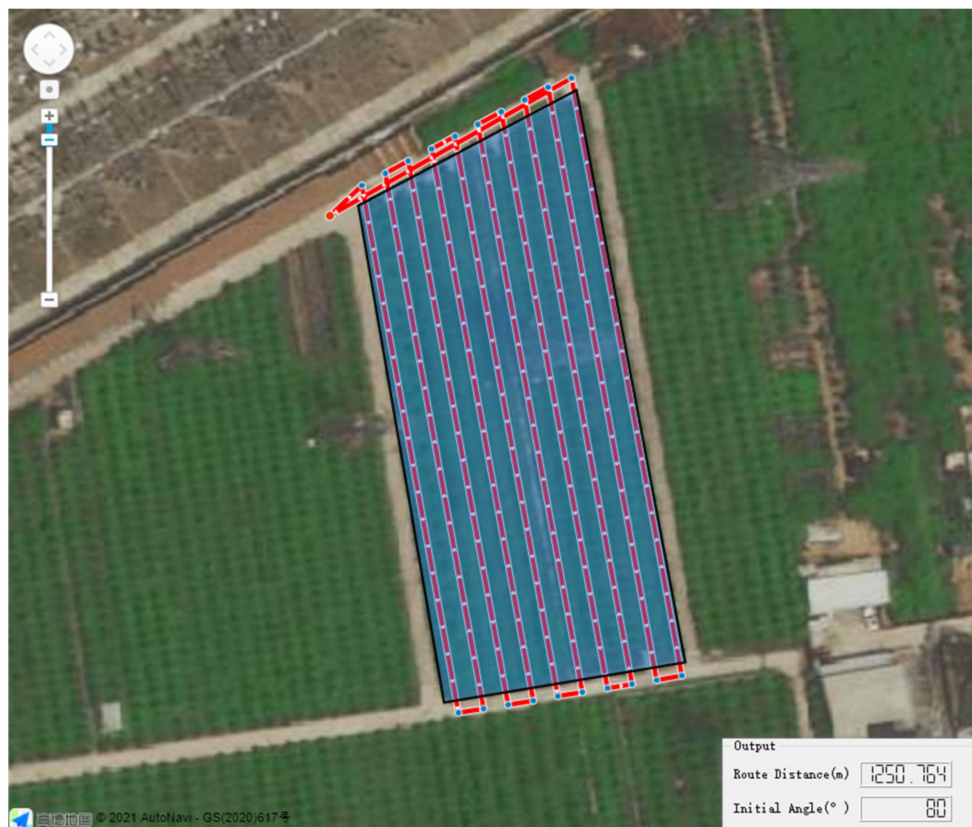
Figure 8. Results of the route-planning simulation software. The red lines with arrows are the calculated optimal route, the blue points are the waypoints, and red point is the takeoff and landing point.
