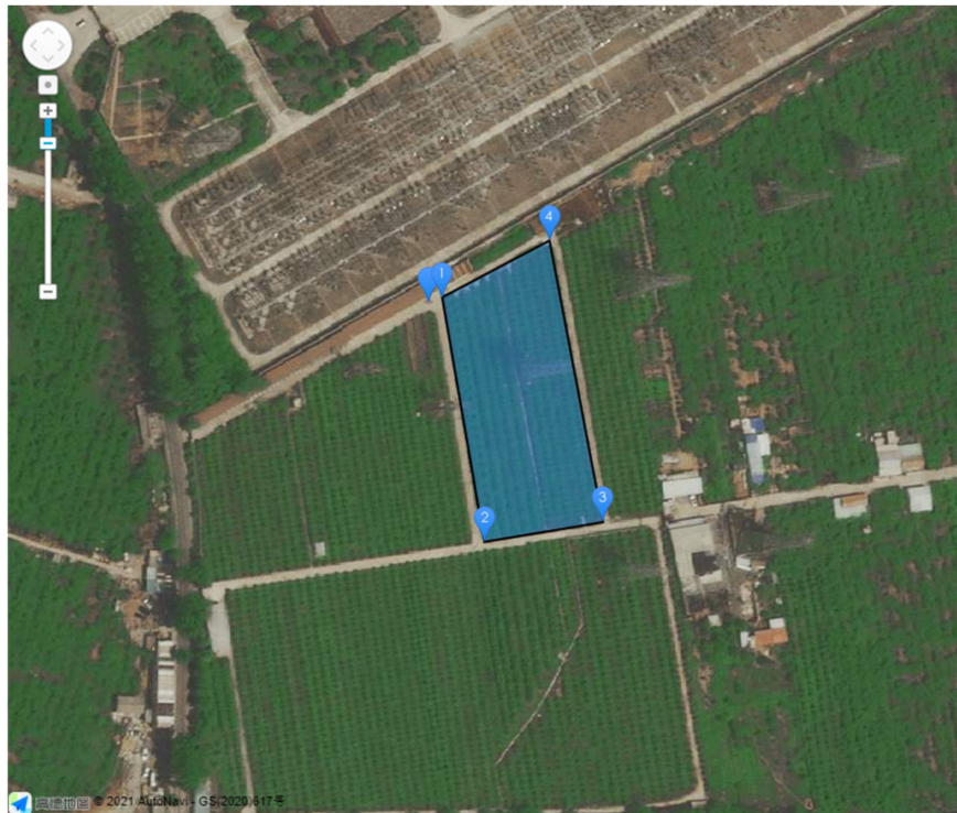
Figure 6. The vertices of the convex polygon operation region and the takeoff point. The unnumbered marker represents the takeoff point, while the numbered markers represent the vertices of the operation region. The blue convex polygon with a black border is the operation region.
