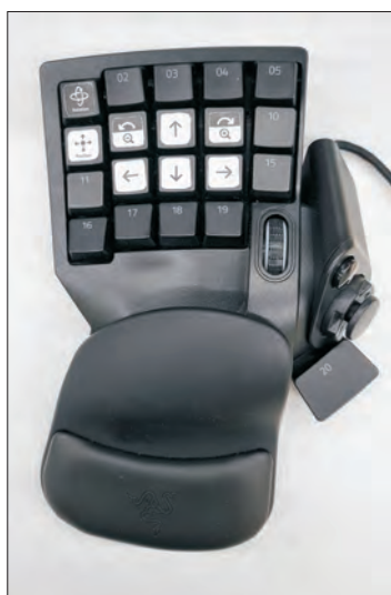
Fig. 2. Controller. The controller designed to allow one-handed manipulation of the augmented reality thyroid model using a custom wireless keypad, with functions for zooming, translation in different directions, and rotation in roll, pitch, and yaw.
