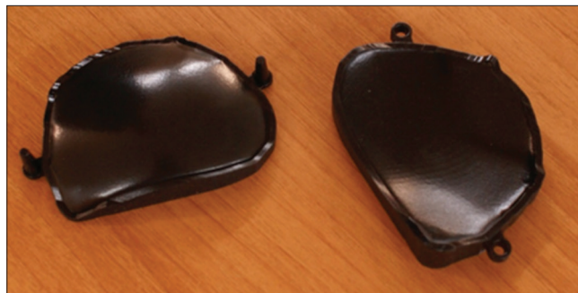
Figure 5: A photo of prefabricated 3D-printed two-piece sterilized silicone mold prepared for the PMMA implant casting.
