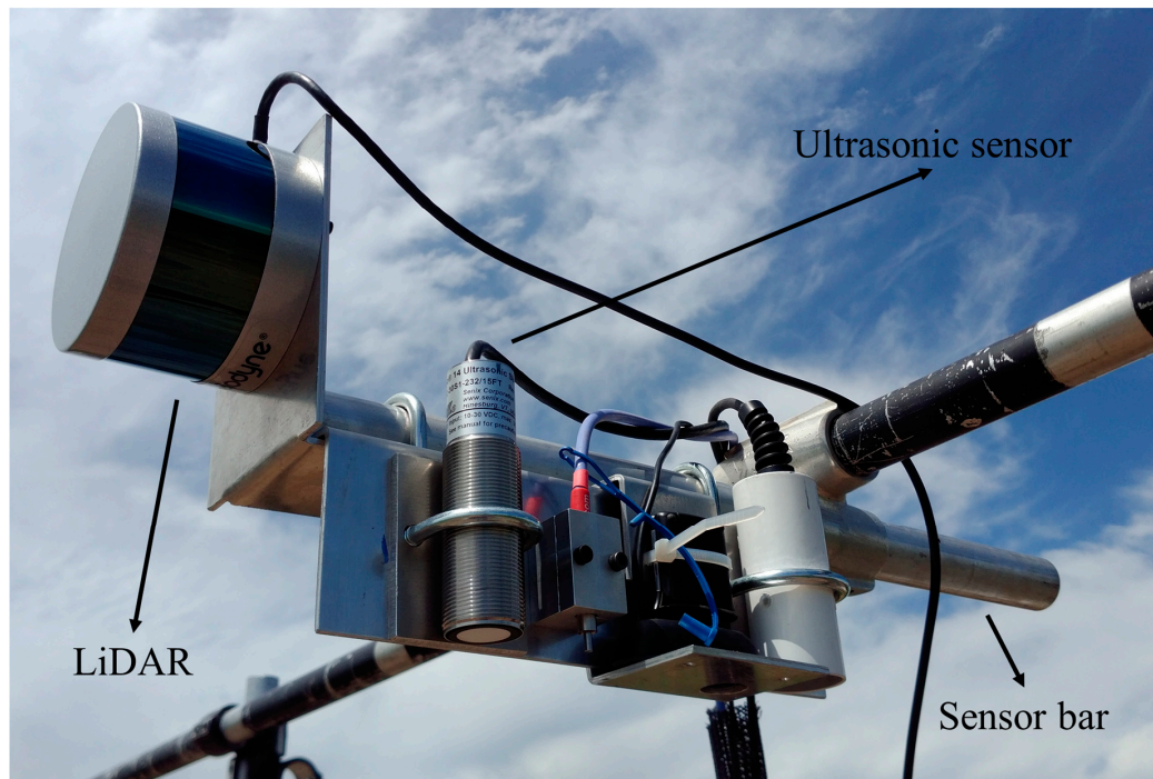
Figure 1. Light detection and ranging (LiDAR) and ultrasonic sensor of the ground phenotyping system.
