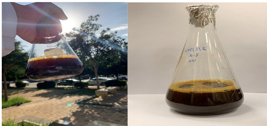
Fig. 1. S. alexandrina leaves extract treated with silver nitrate after 10 min of exposure to sunlight. The dark brown color indicates that the chemical reduction process has been completed.
