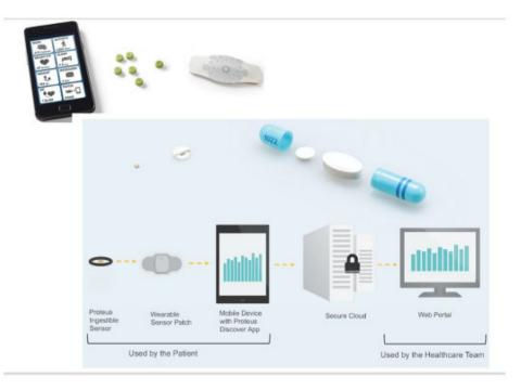
**Figure 7.** Proteus Discover—overview of ingestible sensor system (top) depicting sensor-co-encapsulated pill, a wearable patch, and mobile device app from which stored medication adherence, physical, physiological/ behavioral data are sent to provider web portal from the secure server once pill is ingested (bottom).
