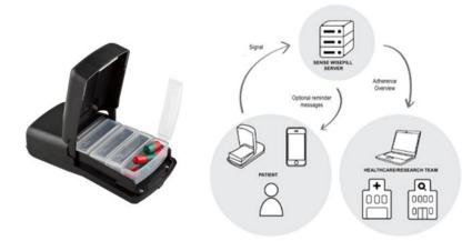
**Figure 4.** Schematic of a pill box – Wisepill RT2000 for medication adherence monitoring. As patients open the box, a cellular signal is sent to the web-based server, and research staff access and transfer the recorded data *via* a centralized server.
