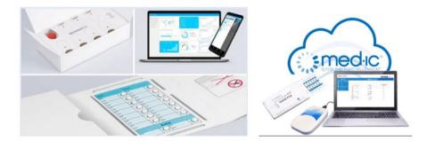
**Figure 3.** Schreiner MediPharm (left) *versus* Med-ic ECM (right). Schematic of the electronic blister pack system showing tablets pushed out from blister pack (equipped with radio frequency identification tag that records medication type, extraction time, specific cavity) and exportation of data *via* smartphone/reader for provider adherence analysis and follow-up.
