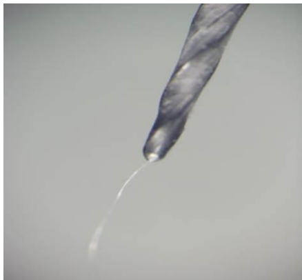
Figure 1. A stereomicroscopic view of wire slivering in F2 ProTaper file (20× magnification)
