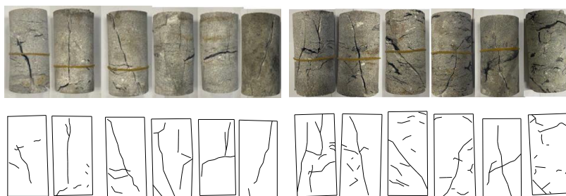
Figure 11. Sketch diagram of failure mode and crack of the coal mixed sandstone sample under triaxial compression.
