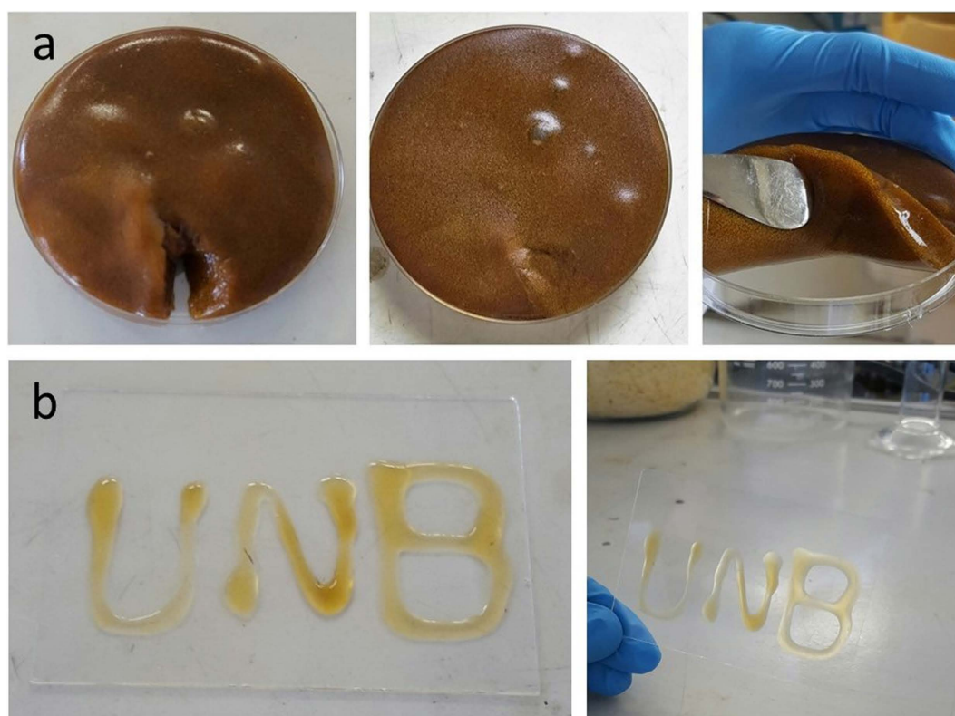
Figure 4. Self-healing and injectable tests. (a) AgNPs/GG hydrogels recovered from a cut without external interventions under room temperature; (b) AgNPs/GG hydrogels were extruded through a syringe directly onto a glass slide, which showed their injectable properties (the AgNPs/GG hydrogels used for injectable testing were prepared using 0.5% (w/v) GG solution).
