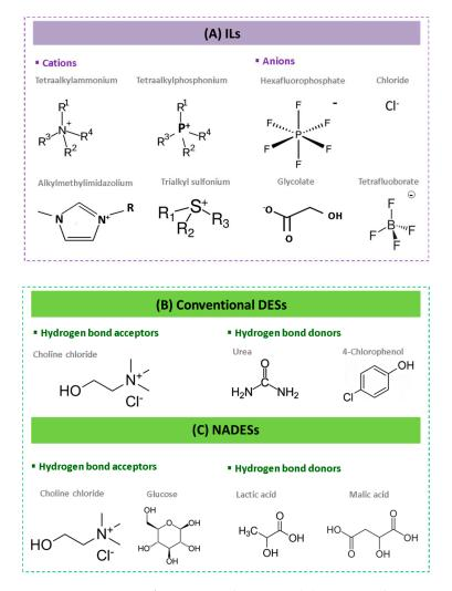
**Figure 3.** Most common components of ILs, DESs and NADESs. (**A**) Cations and anions most commonly used for the preparation of ILs. Hydrogen bond acceptors and hydrogen bond donors most commonly used for the preparation of DESs (**B**) and NADESs (**C**).
