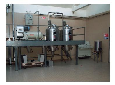
**Figure 6.** Industrial scale ultrasound extraction process ( $2 \times 500$  L) as intensification technique for extraction using vegetable oils (Reus—www.etsreus.com).
