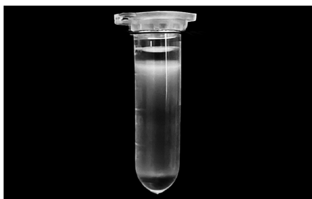
Figure 7. Continuous density gradient centrifugation of post-separation at 48 h
