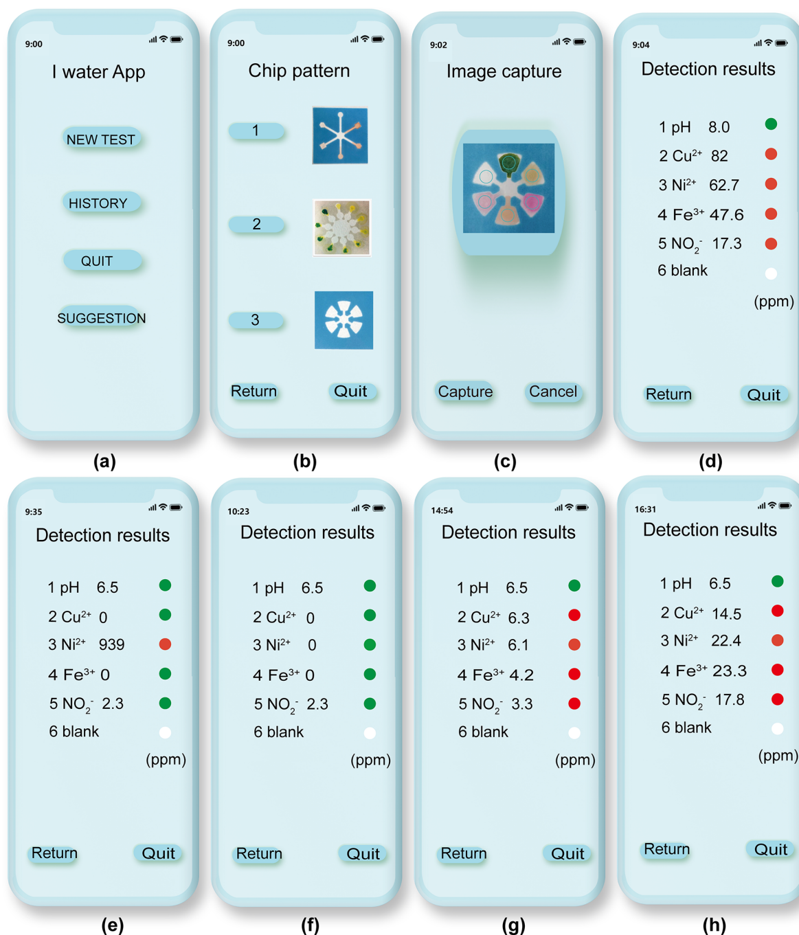
Figure 3. Images for each functional interface of the “I water” smartphone-app. (a) Main menu interface, (b) Chip pattern selection interface, (c) Image capture interface, and (d) Detection result interface. The red dot represents the ion content exceeding the standard, the green dot represents the ion concentration fit for the standard, and the white dot represents the blank control. Results of smartphone app for determination of Cu(II), Ni(II), Fe(III), \text{NO}_2^- , and pH in (e) raw industrial water, (f) purified industrial water sample, and (g,h) spiked river water samples 1 and 2.
