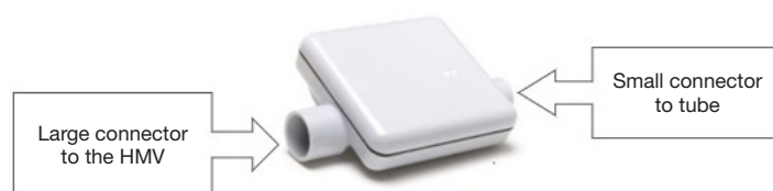
Figure 1 SRETT device, Paris, France. The device is placed between the HMV and the tube leading to the facemask. It measures flow and automatically transmits the data to the hospital. The patient does not need to be present for the attachment of the device to their ventilator. This can be organised with the annual service of the equipment (remotely via the use of a courier). HMV, home mechanical ventilation.
