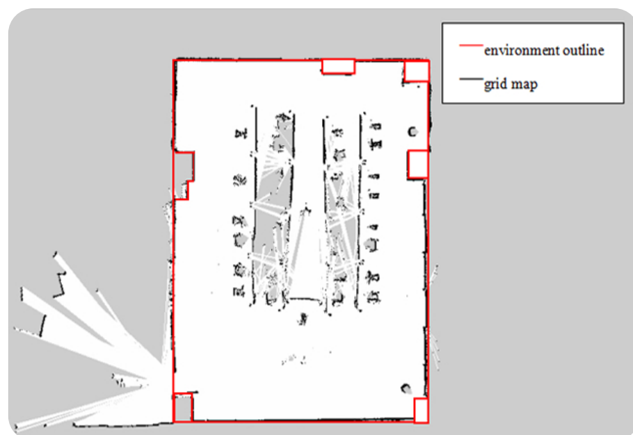
Figure 18. The grid map constructed by the optimized Gmapping mapping algorithm in a small indoor environment.
