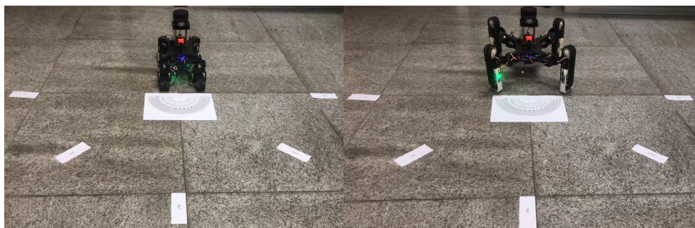
Figure 15. The turning experiment in tracked and legged modes.
