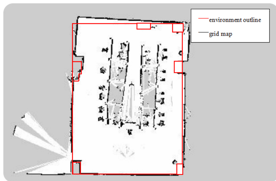
Figure 17. The grid map constructed by traditional Gmapping mapping algorithm in a small indoor environment.
