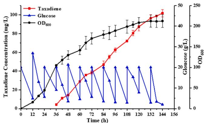
**Fig. 6.** Fed-batch fermentation of metabolically engineered strain M4. Taxadiene production of recombinant strain M6 in batch fermentation. Fermentation was performed in a 5-L jar fermenter containing 2 L of medium.
