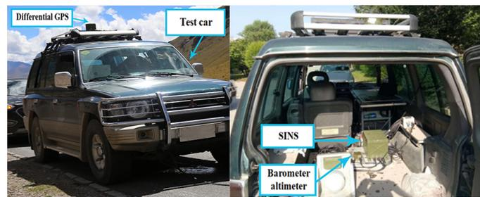
Figure 15. Experimental car and equipment.
