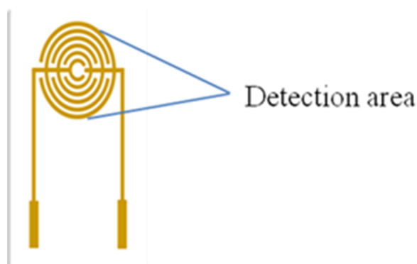
Figure 1 Detection area (droplets area) of the electrode.
